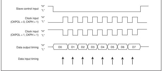
Figure 14.30 Transmission and Reception Timing (CKPH = 1) in Slave Mode (External Clock)
